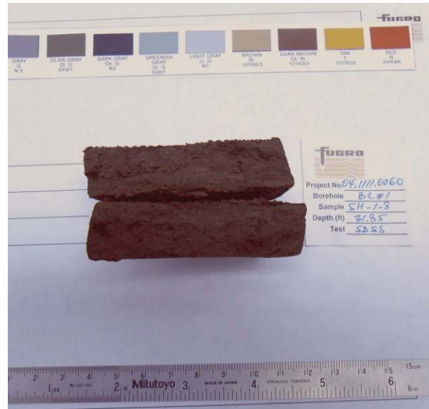
Static Direct Simple Shear Test Boring BH-1 BC#1, Sample SH-1-8a Depth: 31.85 ft. Big Creek Dam #1 and Big Creek Dam #2
