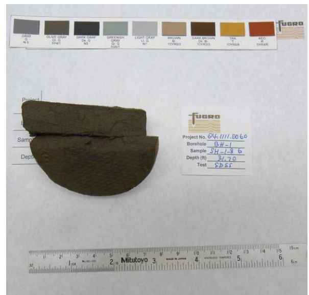
Static Direct Simple Shear Test Boring BH-1 BC#1, Sample SH-1-8B Depth: 31.70 ft. Big Creek Dam #1 and Big Creek Dam #2
