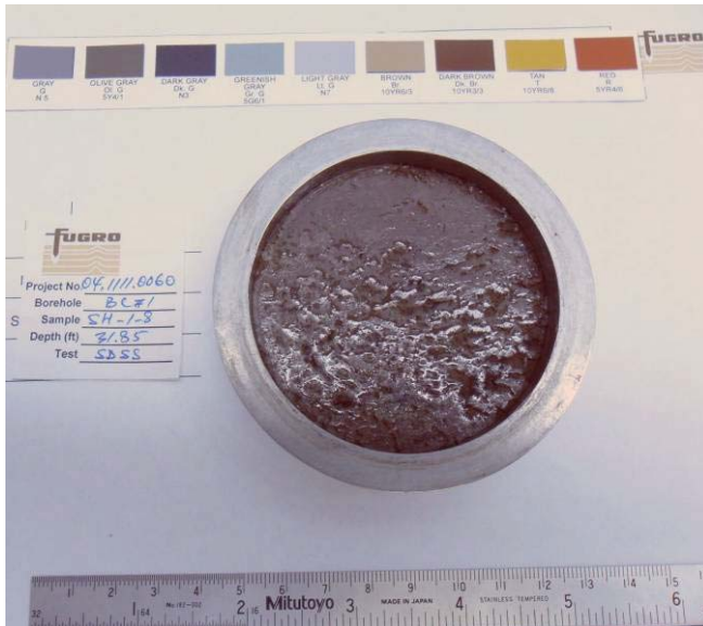
Static Direct Simple Shear Test Boring BH-1 BC#1, Sample SH-1-8a Depth: 31.85 ft. Big Creek Dam #1 and Big Creek Dam #2
