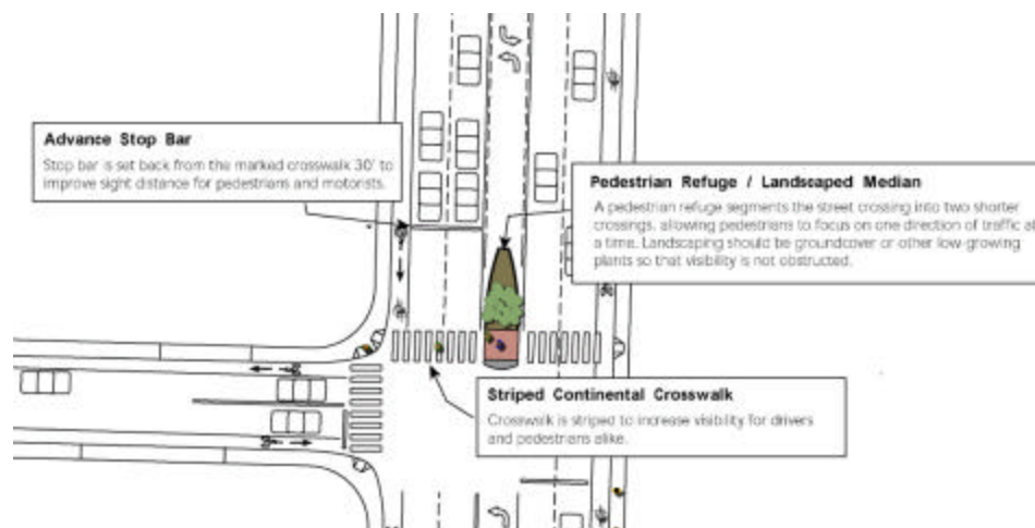
Figure 5-10. Type 1+ Crossing with Median
