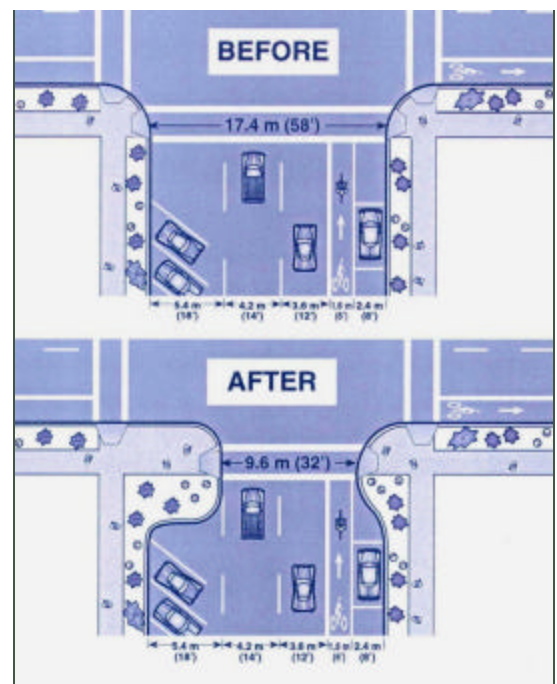
Intersection with curb extensions installed
