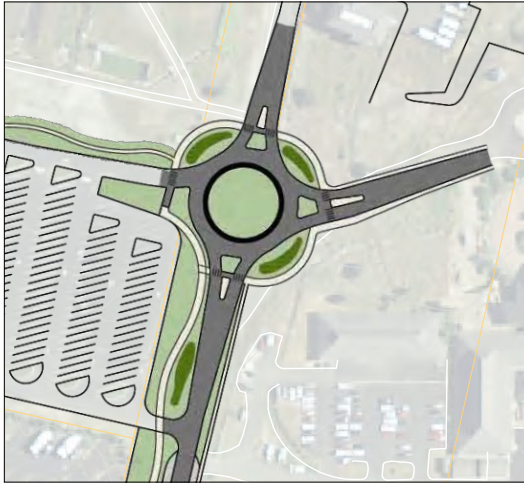
1. Roundabout on SE Marine Science Drive
