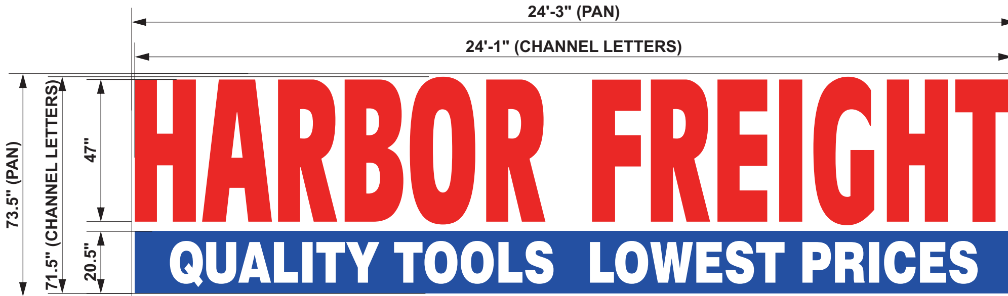
Front Elevation - Sign Type (A) (QTY: 1) Channel Letters - Pan Mounted Scale: 3/8" = 1' (148.5 SQ FT)
