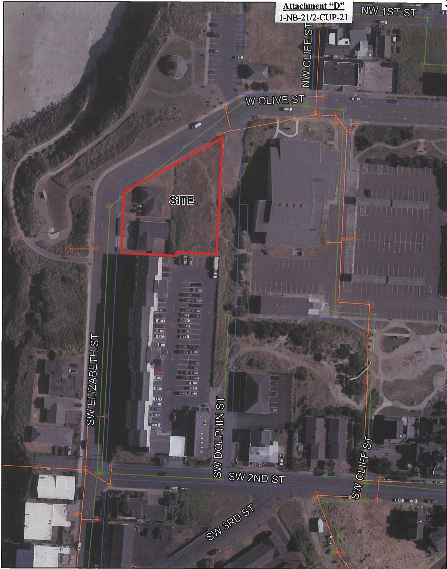
File No. 1-NB-21/2-CUP-21 - Aerial and Utilities (water - blue, sewer - green, storm - orange)
