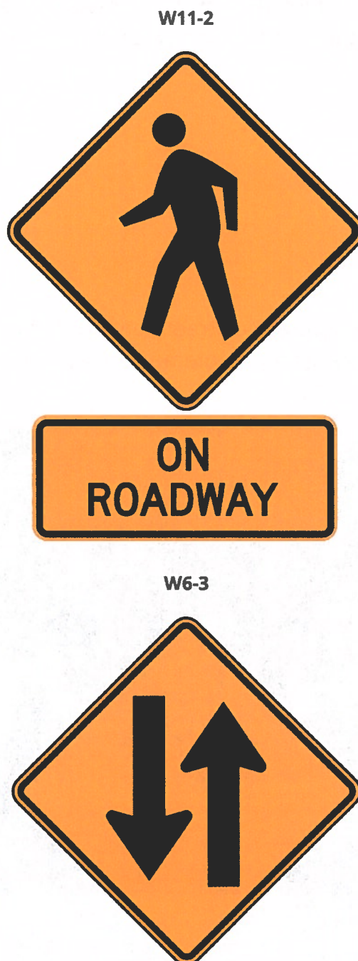
Figure 2-3. Pair a W11-1, W11-2, or W11-15 warning sign with a custom legend plaque to inform road users that shared use by pedestrians and/or bicyclists might occur.
