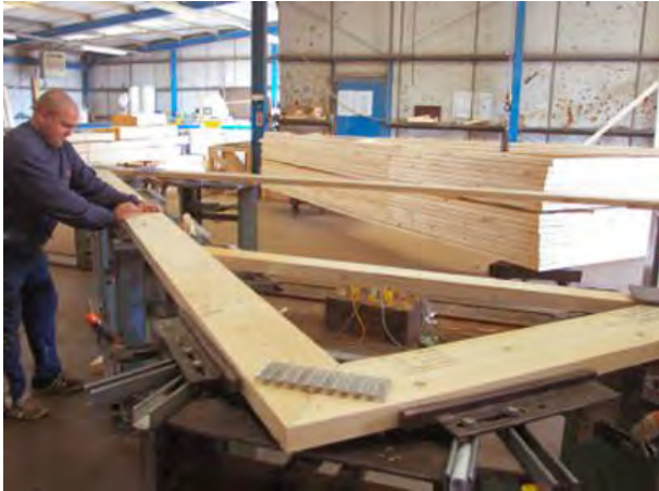
Pre-manufactured trusses are a common form of panelized construction.
