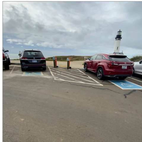
151. Lighthouse Circle parking lot, one-way configuration, 35 regular stalls, 3 ADA stalls (bollards blocking curb ramp), 2 official vehicle only stalls, 2 stalls labeled for compact vehicles, 2 RV stalls, 1 RV/Bus Only stall - Looking West
