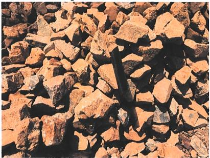
Photo 4 – 3" Open-graded Quarry Stone Fill. Comb shown for Reference.
