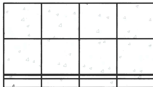
SIDEWALKS 8' AND WIDER SHALL HAVE A LONGITUDINAL CONTRACTION JOINT AT THE MIDPOINT
