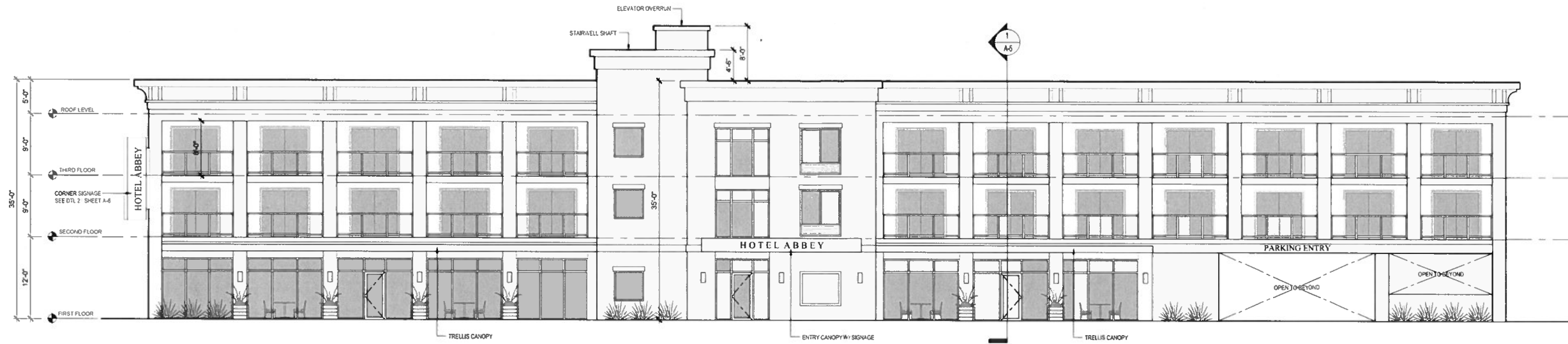
EAST BUILDING ELEVATION (BAY BLVD. FRONTAGE)
