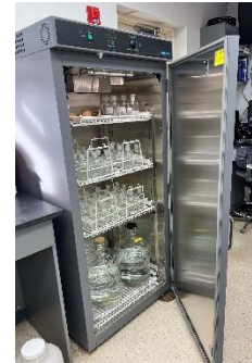
Wastewater Plant Lab Replacement BOD Incubator
