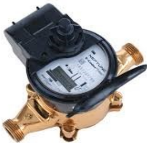
This is the new electronic meter. It will give more accurate reads. Note the digital read window on the meter's face. Also note photo-cell that powers the reading; shine a flashlight on it to activate it.
