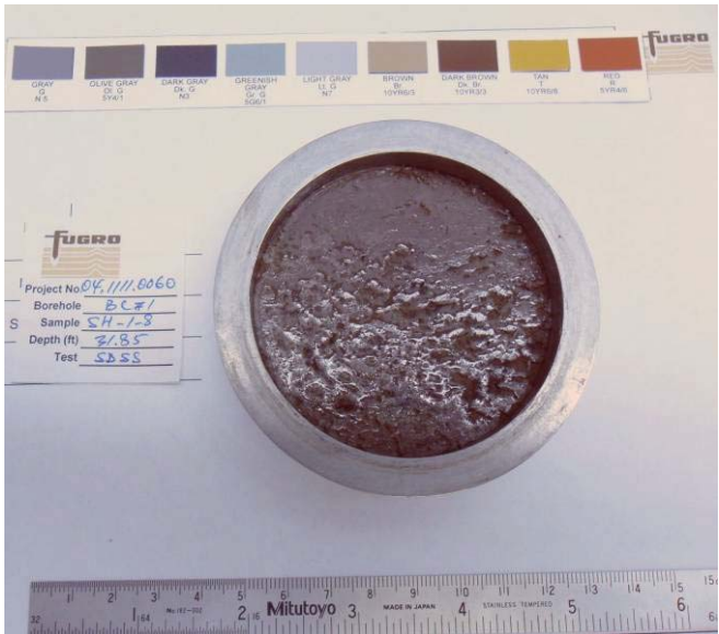
Static Direct Simple Shear Test Boring BH-1 BC#1, Sample SH-1-8a Depth: 31.85 ft. Big Creek Dam #1 and Big Creek Dam #2
