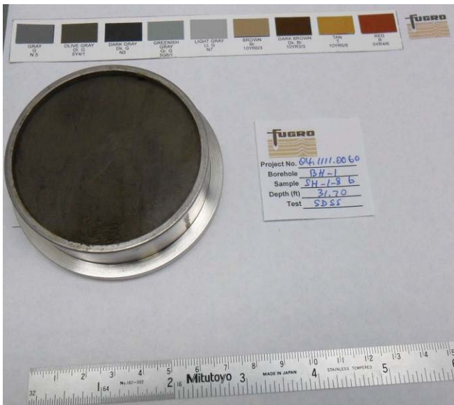
Static Direct Simple Shear Test Boring BH-1 BC#1, Sample SH-1-8B Depth: 31.70 ft. Big Creek Dam #1 and Big Creek Dam #2
