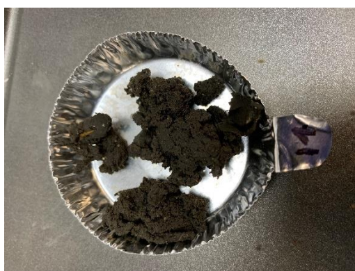
Photo 11 – Polydyne C-6266 15.6 active lb / ton TSS Centrifuge Cake 15 min 3000Gs
