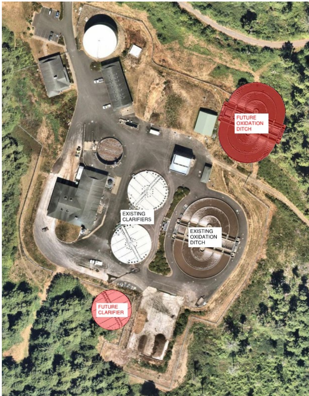
Figure 6-2. Proposed oxidation ditch and clarifier locations
