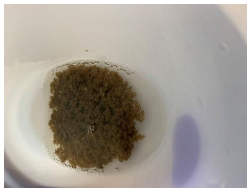
Photo 10 – Polydyne C-6266 15.6 active lb/ton TSS Sheared
