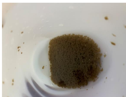
Photo 8 - Plant L-14805 15.2 active lb/ton TSS Sheared
