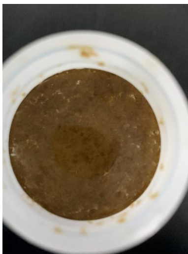
Photo 6 – Floating Floc in Centrate
